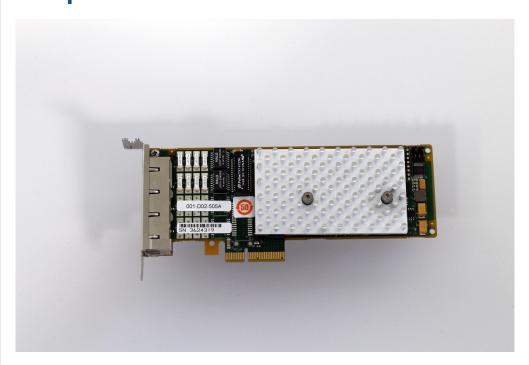
The PCE382 is ideally suited for both PSTN and IP telephony systems that are built on PCI Express architecture and that are capable of handling large volumes of voice circuits for protocol processing transfer to the PCI Express Buses. Application examples include SS7 network elements, wireless infrastructure equipment, media and signaling gateways, and telecom switching and routing equipment.
