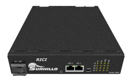
Sunhillo's Real-Time Interface & Conversion Item (RICI) is a versatile and modular platform designed for surveillance and sensor data formatting, filtering, and conversions.
