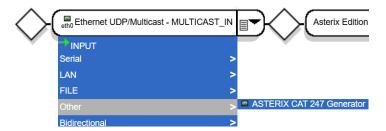
In addition to the message interval (i.e., output rate), the configurable message parameters are: SIC/SAC, Service Identification, and multiple ASTERIX category/version entries.
